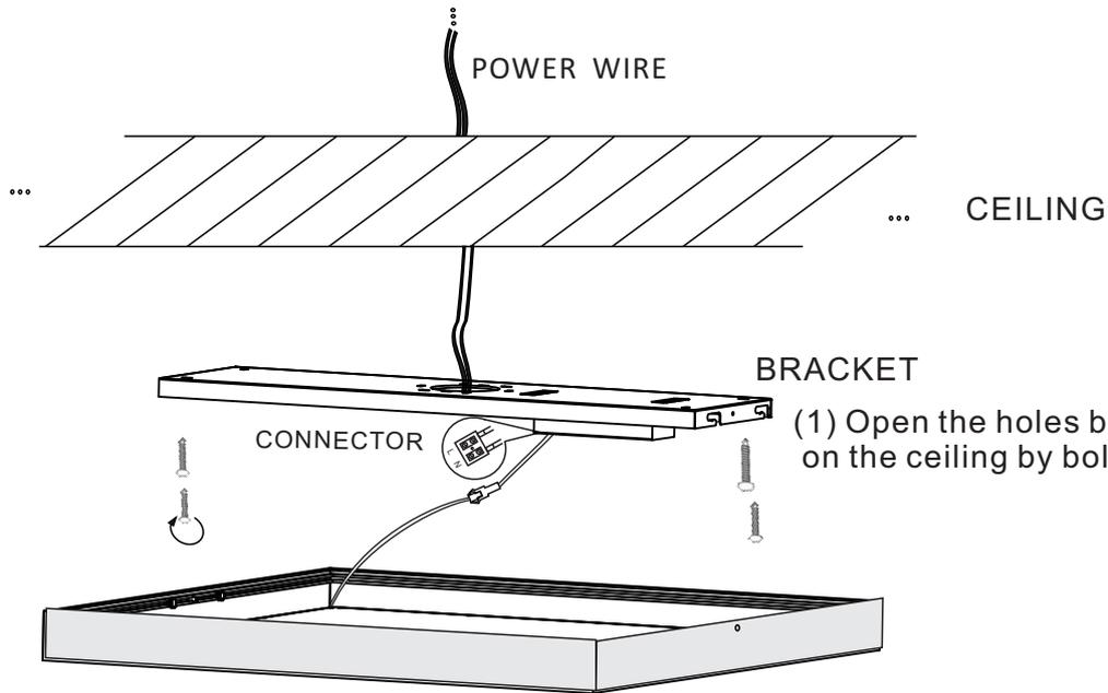
(1) Open the holes by plier, and fix the bracket on the ceiling by bolts.
